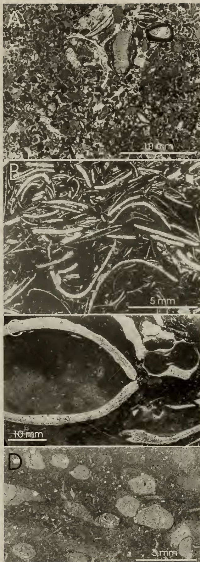
Figure 2 RIGHT. Thin sections of parent limestones in the Daylesford Limestone. A. Skeletal grainstone, from the Manooka Limestone Member, composed dominantly of crinoid ossicles, and subordinate mollusc and coral fragments (USGD 46711). B. Skeletal packstone, from the Ranch Member, composed dominantly of molluscs (USGD 46673). C. Skeletal wackestone, from the Bourimbla Limestone Member, composed of gastropods and the brachiopod Eodinobolus (USGD 46651). D. Burrowed lime mudstone, from the Ranch Member (USGD 47034).
